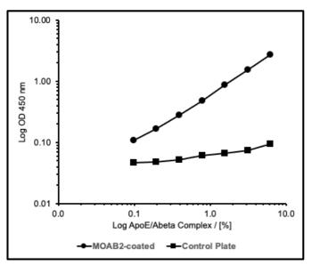
In the above example graph, ApoE/A $\beta$  complex standards were run following the assay protocol. The TMB reaction was stopped after 9 minutes.
