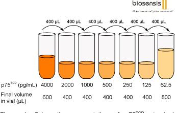
Figure 1: Schematic representation of  $p75^{\text{ECD}}$  standard preparation
